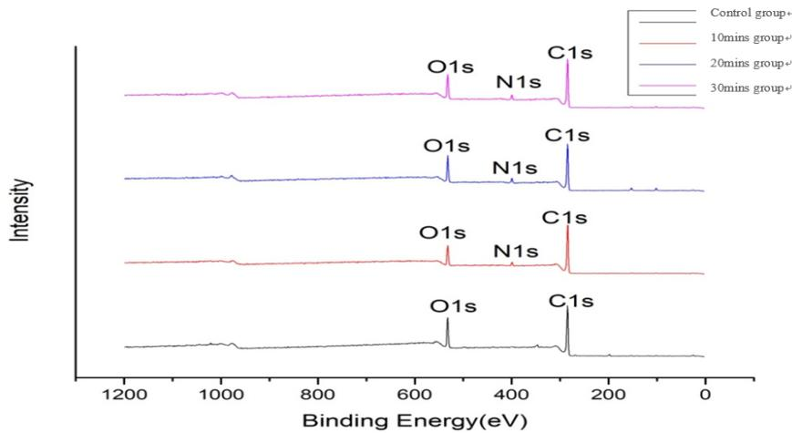
Figure 2. XPS elemental analysis full spectrum of PEEK samples in each group.
