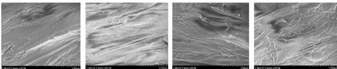
Figure 1. PEEK specimen surface morphology after ammonia plasma treatment (×1000 times).
